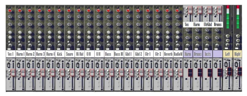
This mixer has got the channel gains (at the top) turned approximately half way around, and all faders up around their zero mark (unity gain). This will mean that, from an electronic point of view, the mixer will be operating correctly. The sign of this will be a healthy electrical level on the output volume meters (the mixer manufacturer assumed you know all of this, and calibrated the mixer accordingly).
