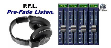
An important tool is the PFL. Use a headphone that has a large diaphragm so that you can hear frequency content properly (small diaphragm headphones have poor frequency response) because you make decisions with the Equalisers based on what you hear. Headphones that are "noise-cancelling" are best suited. Always be listening for the characteristic sound of 'feedback'... it is a bright metallic sound. You can often hear it in the headphones quite easily.
